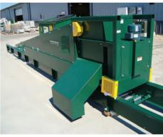
**TRIPPER WITH INDEXING SHUTTLE CROSS CONVEYOR** Tri-Roller design with motorized ear corn letdown assembly.
