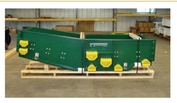
**IN-LINE BELT TRIPPER** Stationary in-line belt tripper for horizontal to incline conveyor changes where space for typical outside arc conveyor wedges is not available.
